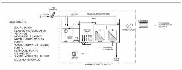
Figure 3-2: Typical MBR Process Flow Diagram
